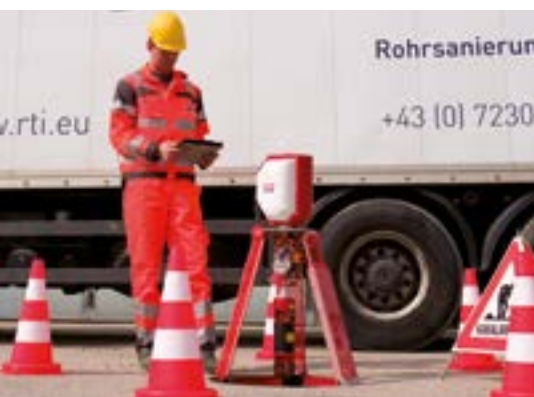
Inspection of shafts with scan technology
