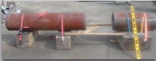
16 inch (400 mm) diameter steel pipe with a 24 inch (600 mm) long piece missing
