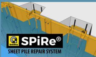
The Sheet Pile Repair or SPIRe® system made exclusively by QuakeWrap is constructed with **lightweight** honeycomb or 3D fabric sandwiched between sheets of **resin saturated FRP fabric**. These panels may be custom prefabricated to match the shape of the steel bulkhead or concrete seawall being repaired.
