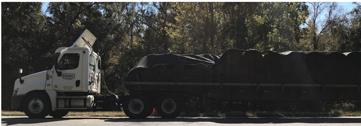
Figure 5: Strain testing with loaded 83,620 pound 18-wheeler
